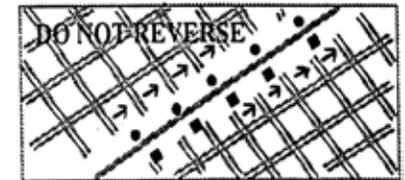
**Matching of side to end seams (1/4 turning) or seams where the middle of a sheet width is positioned against a factory edge is not recommended or warranted. Factory edge overlap of more than 3" is not recommended or warranted.**
