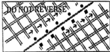
**Matching of side to end seams (1/4 turning) or seams where the middle of a sheet width is positioned against a factory edge is not recommended or warranted. Factory edge overlap of more than 3" is not recommended or warranted.**
