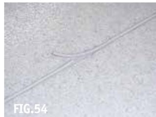
If the temperature is set too high or the welding speed is too slow, burning of the flooring may occur. If the temperature is set too low or the welding speed is too fast, poor adhesion of the weld thread to the flooring may occur.
