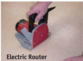
> When using a contrasting colored weld thread, all seams must be routed with an electric router.
