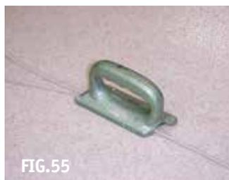
**FIG.55:** The use of the seam plane is the preferred and recommended method for trimming heat weld thread.
